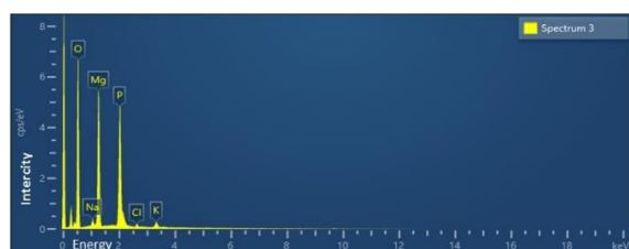
Figure (3-4) EDS analysis of MgO NPs synthesized by B. subtilis .
