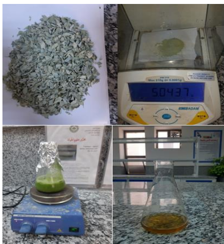
Fig. 2: Steps Preparation leaves extract of Atriplex nummularia
