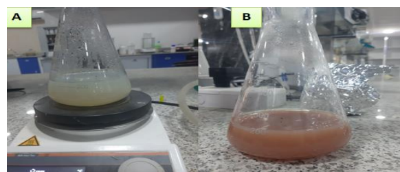
Fig.3. Formation of green silver nanoparticles(a)during add leaves extract(b)after 24 h.
